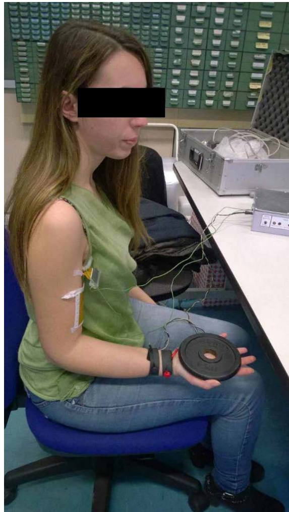
Figure5.4: Position and task of the subject during HD-sEMG acquisition. The subject was asked to sit down with back on the chair and hold 3kg weight with her palm up without touch the leg for 5 seconds.
