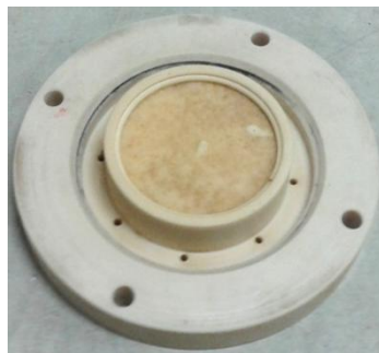
Fig 5.5 – Sinterized glass distributor
