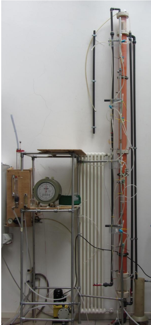
Fig 5.3 – Bubble column reactor
