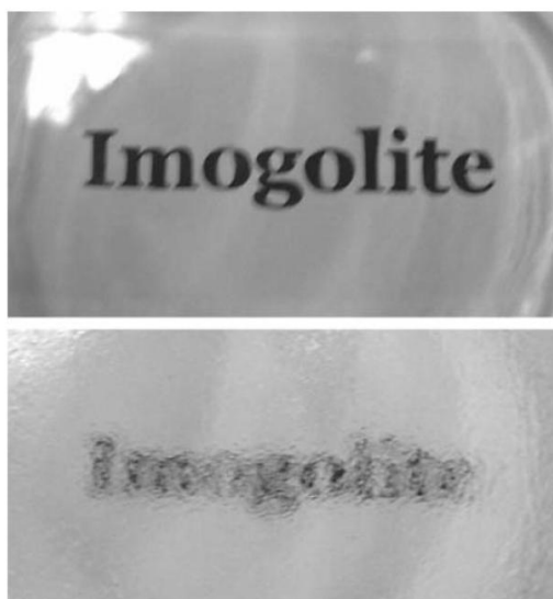
Fig. 15 Transparency of in situ hybrid (upper) and blend (lower) imogolite/PVA films. The thickness of films is ca 100 \mu m. Imogolite shows to be optically transparent in the multilayer film [286].
