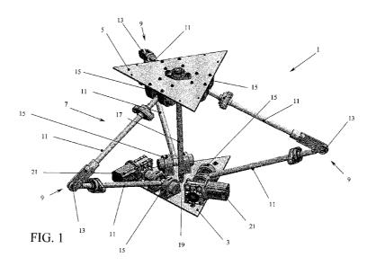
(57) Abstract: A sun follower (1) is described, composed of at least one fixed supporting base (3) and of at least one moving structure (5) controlled and adapted to support at least one photovoltaic module, between such fixed supporting base (3) and such moving structure (5) actuating means with parallel kinematics (7) being interposed, adapted to handle such moving structure (5). A process for controlling such sun follower (1) is also described.
