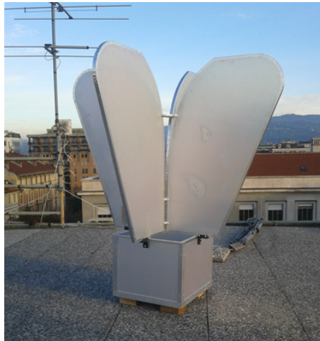
Figure 6.9: Prototype of the Vivaldi v3.1 on the IEIIT-CNR roof, for the reflection coefficient measurement.
