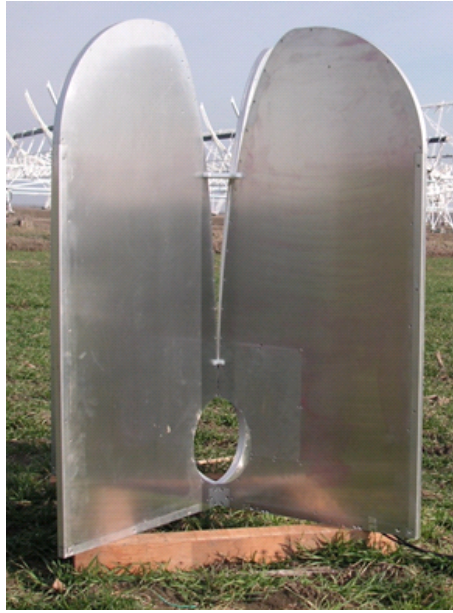
Figure 6.2: Prototype of the Vivaldi v2.0 antenna realized by IRA-INAF.
