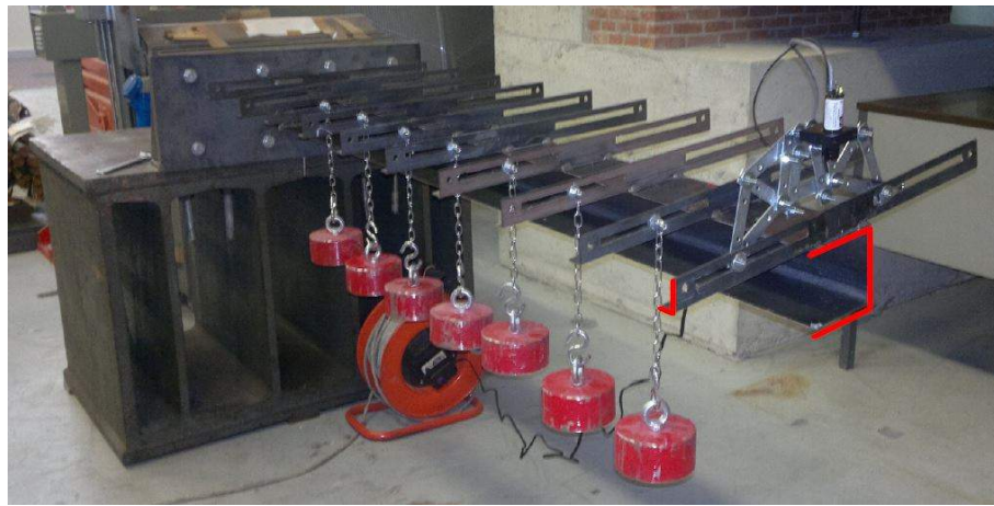
Figure 3.18 – Application of the external concentrated loads.
