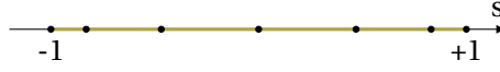
Figure 1.2: The reference element \tilde{\Omega} in 1 dimension, with the internal positioned according to the GLL formula with K=6 .
