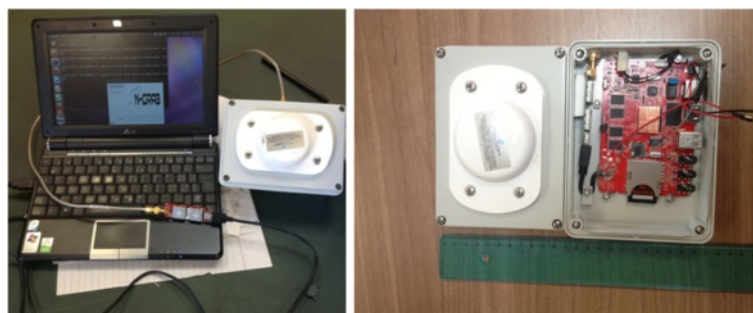
Figure 2 Prototypes of the GNSS-R receivers developed. PC-based solution (left panel). Hackberry board connected to the SiGe radio frequency front end (right panel).
