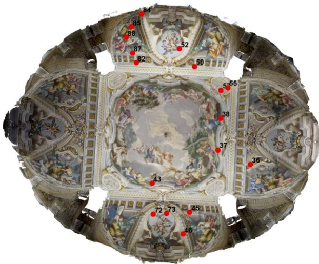
Figure 5 GCP used for bundle block adjustment
