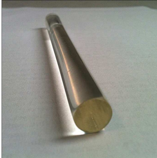
Figure 3.5: Photograph of a core rod after polishing
