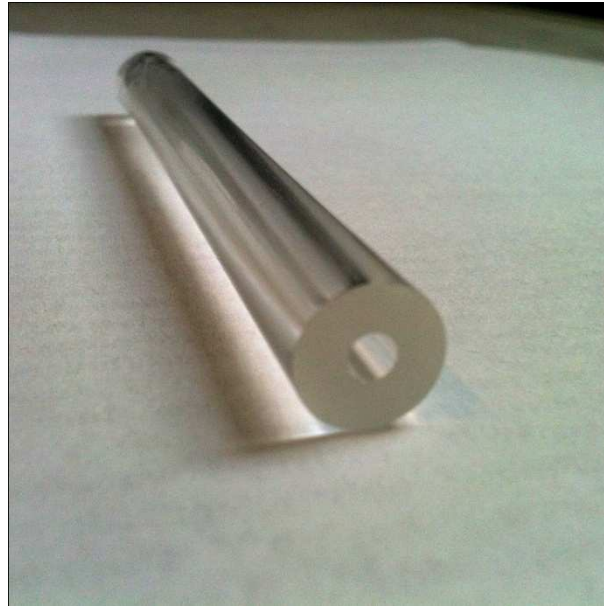
Figure 3.8: Photograph of a cladding tube after polishing
