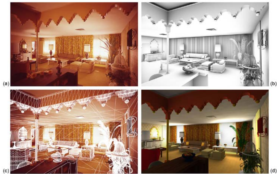
Figure 52. (a) A historical photo of one of the Aqueduct suites, which can be compared with its 3D reconstructed version (b). The accuracy thereof can be appreciated from the superimposition of its wireframe model on the original image (c). Finally, a daytime photo-realistic rendering of the virtual suite is shown in (d).
