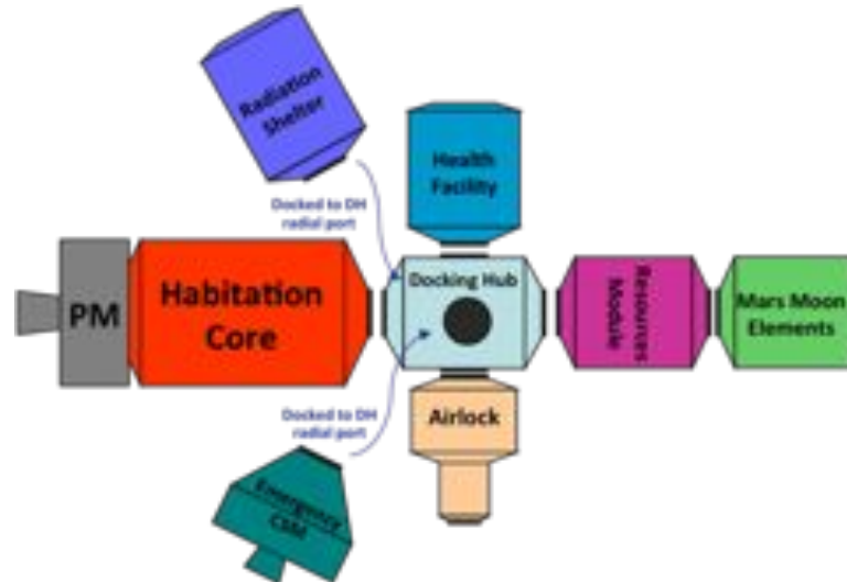
Figure 7.13: Mars Moon outpost configuration (not in scale)
