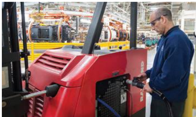
Figure 1.8. Fuel cell powered forklift during the re-fuelling operation [14]. The average re-fuelling time is around 3 minutes against the 8-10 hours of re-charging time of a traditional battery powered forklift.
