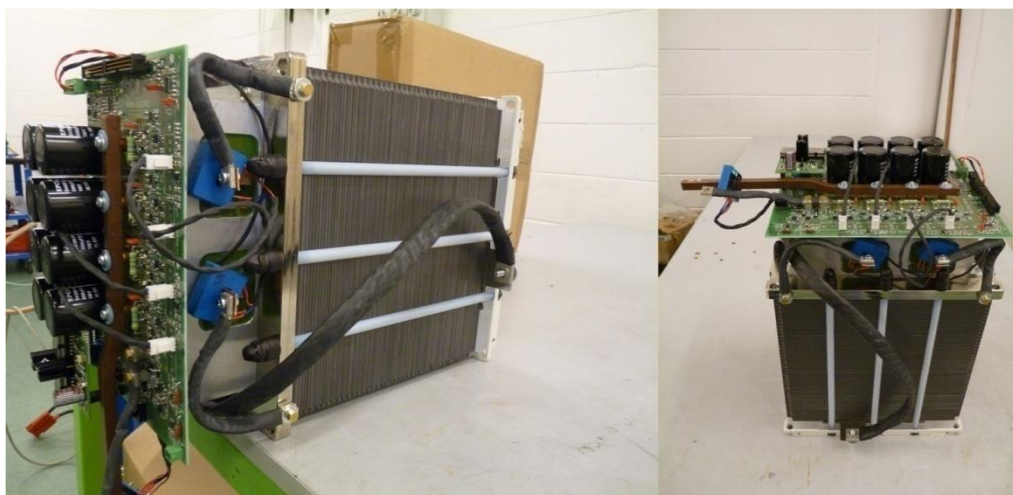
Figure 4.4. Picture of the first prototype implementing the DC-DC thermal and electrical integration with the stack.
