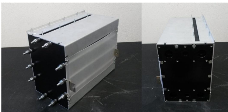
Figure 1.2. 56-cell PEM fuel cell stack assembled by Electro Power Systems.
