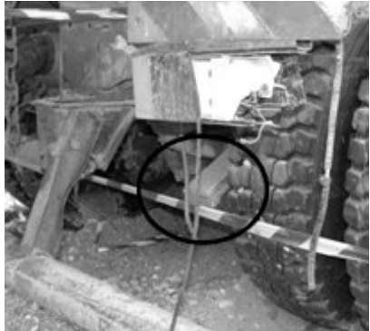
the couple of collapsed leaf springs
