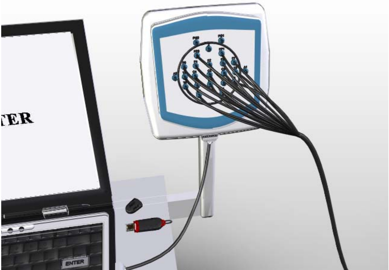
Figure 6. Electrodes connection to the amplifier
