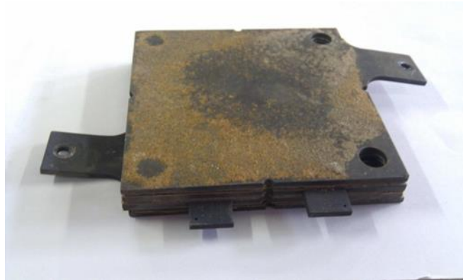
Figure 5-14: STACK 1 after the disassembly
