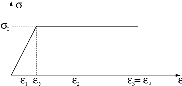
Figure 9: Example illustration of the strain distribution in the tension rings and associated stress state according to elastic-plastic constitutive law.
