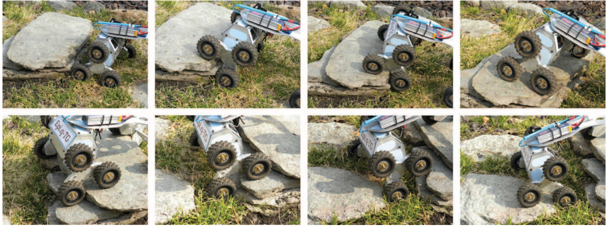
Fig. 13. Epi.q-2 negotiating an obstacle
