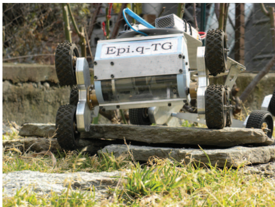
Fig. 17. Epi.q-2 traversing an obstacle, on uneven ground
