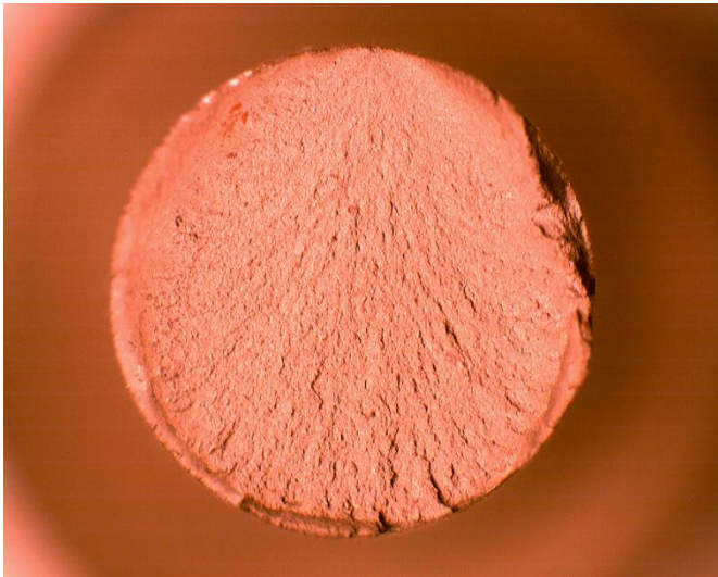
Hipped tensile test sample (shear lips presence)
