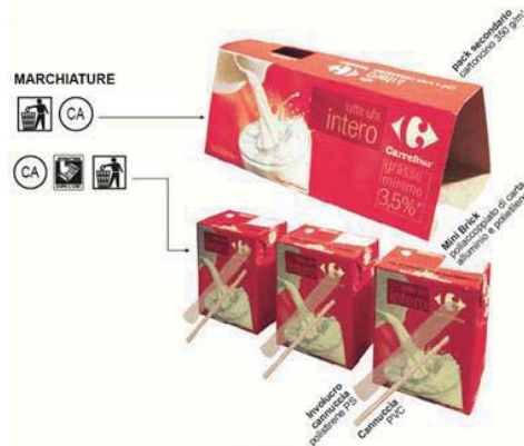
Figure 3: Example of an exploded view of a milk packaging
