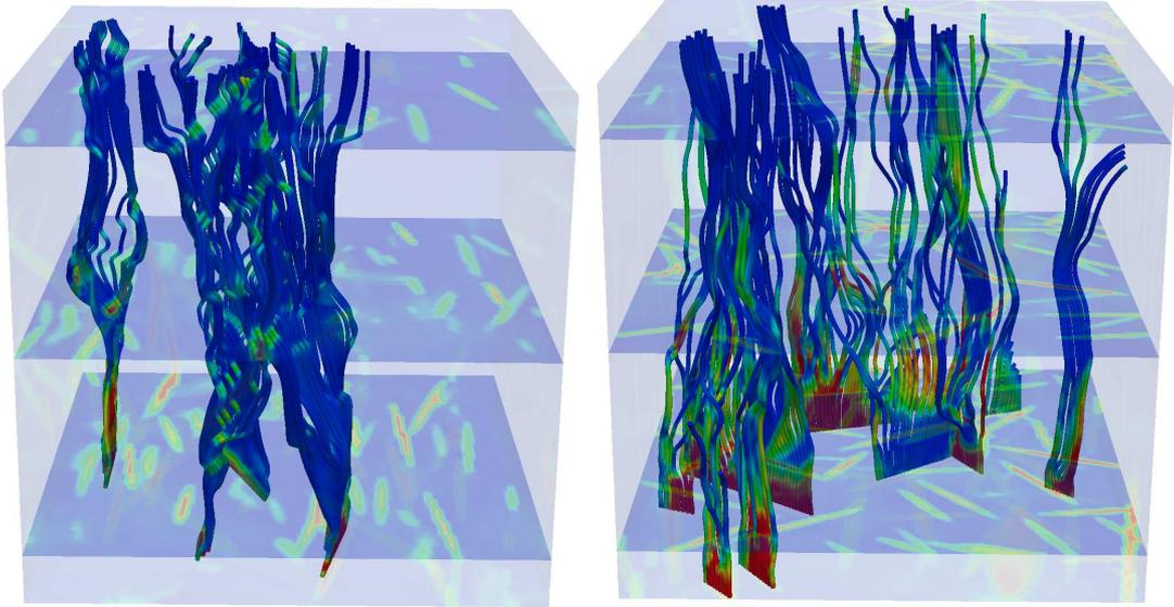
Figure 8: (Color online)  $Y_f = 0.298$ ,  $k_f/k_p = 36.5$ . Left-hand side: Streamlines of the heat flux along percolating paths, where the extrusion axis is aligned with the  $x$ -axis. Right-hand side: Streamlines of the heat flux along percolating paths, where the extrusion axis is aligned with the  $z$ -axis. Colors provide an indication of the heat flux intensity.
