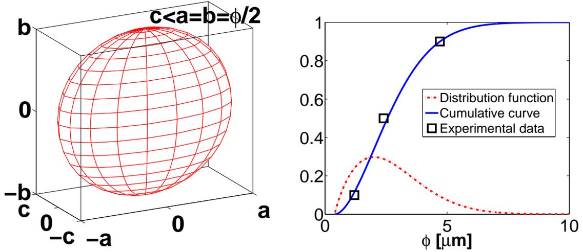
Figure 4: (Color online) Left-hand side: Graphite particles are modeled as oblate ellipsoids. Right-hand side: The ellipsoid size  $\phi$  follows a distribution function (dashed line) reconstructed on the basis of cumulative experimental data (squares). The corresponding cumulative curve is also reported with a continuous line.
