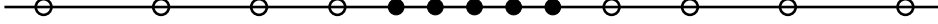
Fig. 3. Illustration of stretched mesh in one dimension. The grid spacing between two adjacent disks is \Delta x = \delta_x = 1 , and that between two circles or a circle and a disk is \Delta x > \delta_x = 1 . For nodes indicated by circles, interpolations are necessary to compute the data \{f_i\} after advection.
