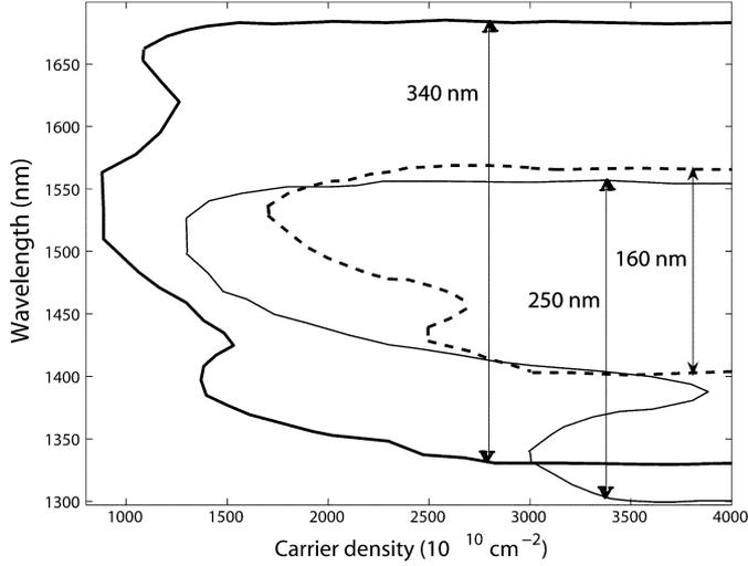
Fig. 6. Optical gain bandwidth calculated for  $g_{th} = 7 \text{ cm}^{-1}$  and using the single isolated dash model (solid line) and the dash coupling with WL model (dashed line). The thick solid line is the bandwidth of the QDash structure designed in Section III-C for very broad optical bandwidth. At a fixed carrier injection, the bandwidth ( $g_{net} \geq g_{th}$ ) is the wavelength range limited by the each curve.
