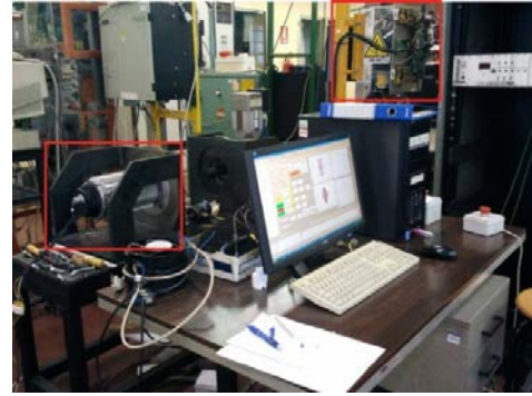
Figure 15. Setup #2. The dSPACE 1104 R&D host computer is visible on the desk. The PM-SyR machine under test and the inverter are in the red squares.
