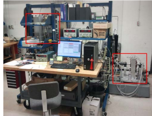
Figure 14. Setup #1, used for the IPM and the SPM machines. The dSPACE 1103 PPC host computer is on the desk. The machine under test is in the red square at the bottom right corner, connected to an induction machine dyno via a torque-meter (not visible). Power converters are in the other square on the left hand corner.
