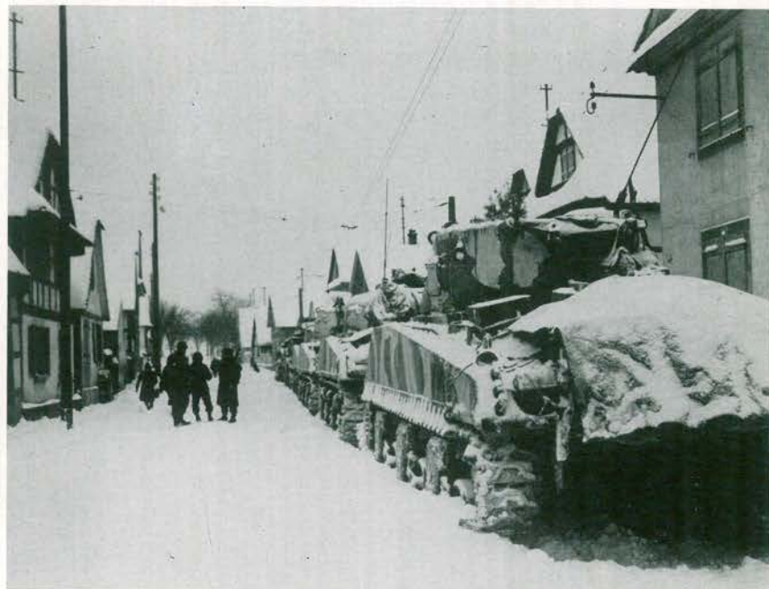
M-4 tanks mounted with 75mm and 76mm, camouflaged with white paint and whitewash, line up in Oberschauffolsheim, ready for a new attack.
