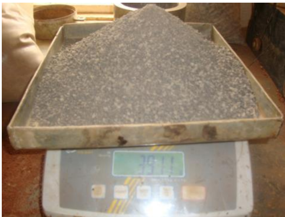
Fig 2; Clay soil on weighing balance
