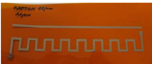
Fig. 8. Meander inductor on flexible Kapton substrate.
