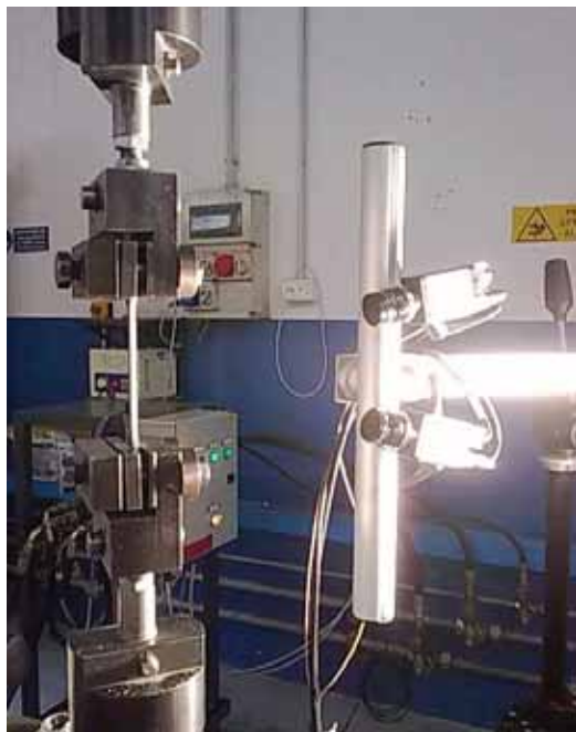
Figure 7. Performing experimental (tensile) tests
