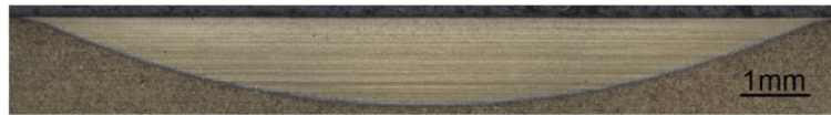
Fig. 3. The macrostructure of the surface hardened area in a perpendicular direction - field deflection. (full colour version available online)
