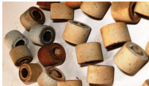
Fig. 3. Alumina coated specimens damaged due to slurry erosion [49]
