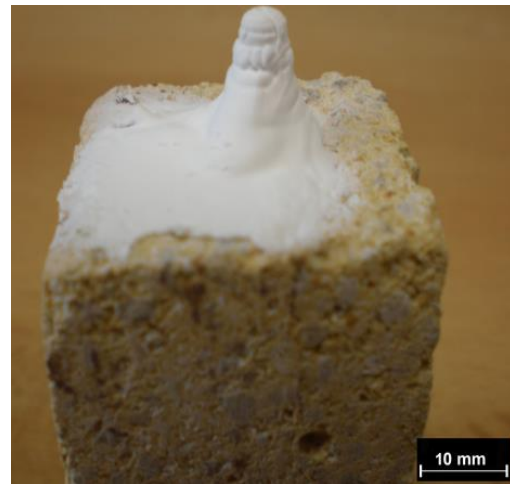
Fig. 2. Formed zinc oxide on the surface of chamotte. (full colour version available online)
