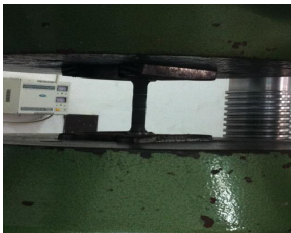
Fig. 6. Tensile test being performed on UTM. (full colour version available online)
