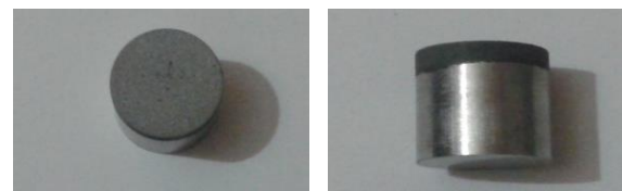
a) Micro Vickers hardness test specimen
