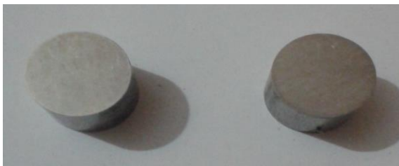
Fig. 1. Specimens for Micro hardness test.
