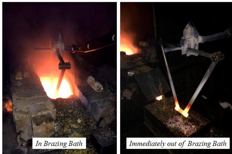
Fig. 7 Dip brazing of head joint. (full colour version available online)
