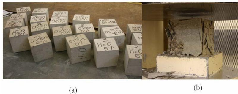
Figure 1 (a, b). Testing compressive strength of concrete specimens: (a) specimens before testing; (b) after testing
