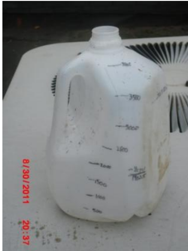
Figure 17: Standard milk jug used for watering. The handwritten lines were approximations of fluid volume as measured by a graduated cylinder.
