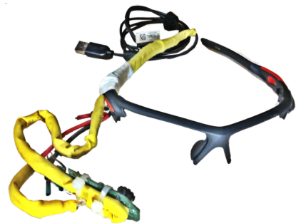
Figure 1: The DIY eye gaze tracking glasses result.
