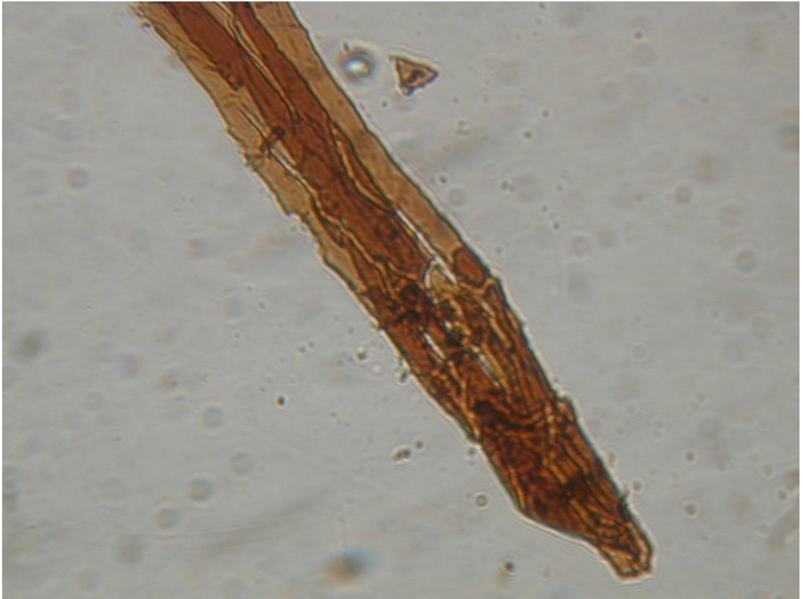
Figure 7.14. Ultimate fiber, showing thick cell wall, thin lumen, and tapered natural end
