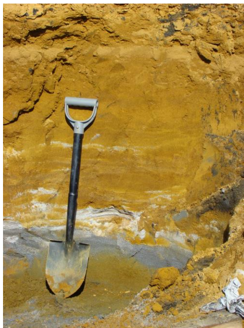
Fig. 5. Vertical cross-section of oxidized Camp tailings from the Sherridon Mine. Oxidized zone with discontinuous Fe(III) hardpan (reddish-brown) overlying continuous Fe(II) hardpan (white and gray-blue). Shovel is approximately 0.7 m long.
