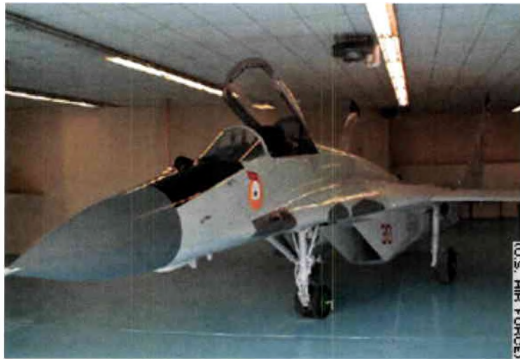
Figure 25: MiG-29 with Slotback radar (not seen because it is within the nose radome) and IRSTS that is shown as a black protrusion just below the front of the canopy.
