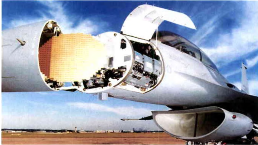
Figure 24: Picture of an actual APG-68 v9 radar. A notional APG-68 radar capable of detecting turbulent wakes may look similar.
