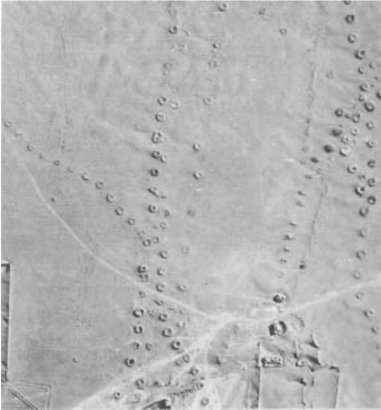
Figure 4 Qanats Converging on the City of Kirman. Built during the course of many centuries, large numbers of qanats converge on most Iranian Plateau cities. Some of these old qanat tunnels cross back and forth between channels, others are twin qanats one or both of which may be active, and many have been abandoned. No map of the resulting labyrinth of qanat tunnels is available. Note the differences in surface definition on the image caused by drifting sand.
