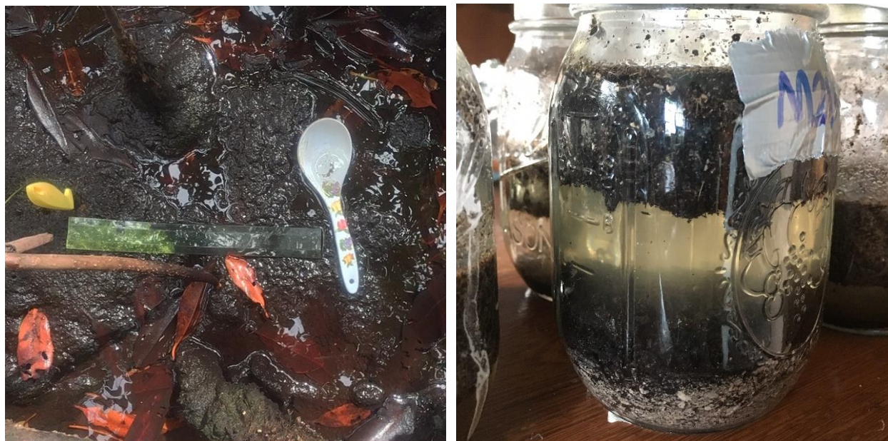
Figure 3: (Left) Mangrove sediment sample collection process; (Right) A mangrove sample during the first flotation process to remove sediments
