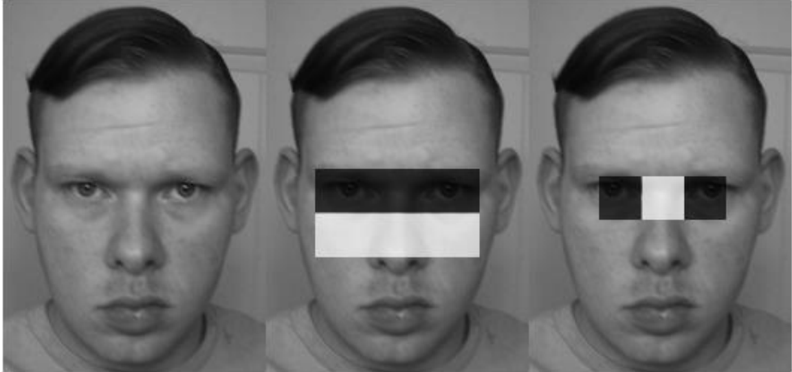
Figure 4.5 – The left image is the input grayscale intensity image. The middle image shows a Haar cascade classifier feature used for distinguishing between the eyes and cheeks of the frontal face. The right image shows a second Haar cascade classifier feature used for further distinguishing the presence of eyes on the frontal face image.
