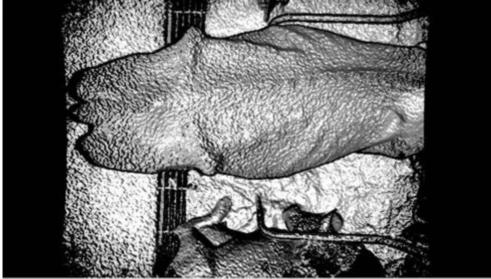
Figure 5.6 – Kinect Studio in “Surface with Normal” image mode for the depth frame.
