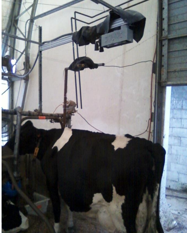
Figure 5.2 – Respiration rate monitoring system viewed from beside the cow with the system operating above the cow.
