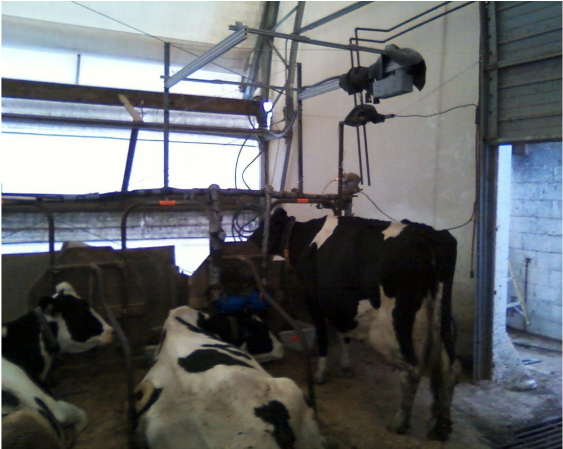
Figure 5.1 – Respiration rate monitoring system viewed at an angle from the cow with the system operating above the cow. The current system is capable of expanding to include a second monitoring camera above the middle cow in the image.
