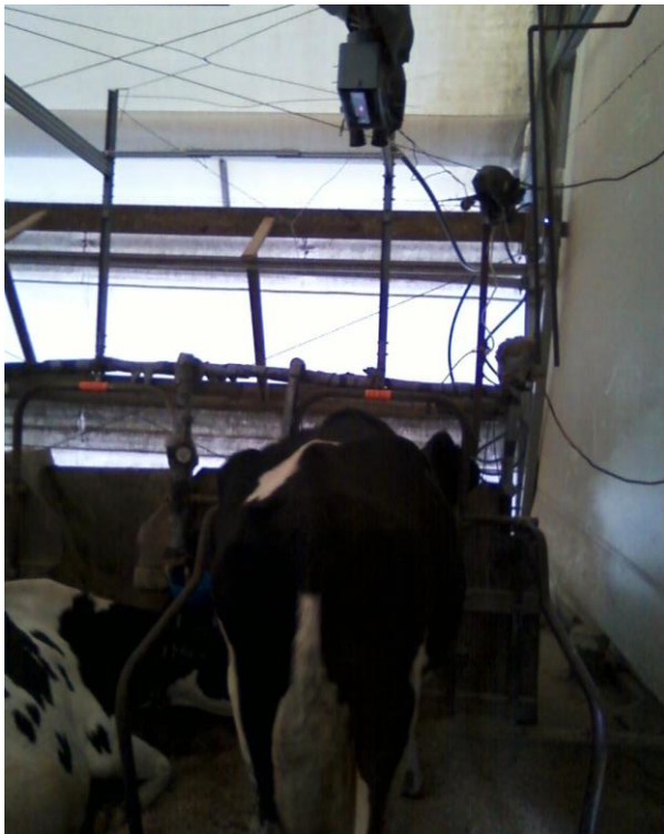
Figure 5.3 – Respiration rate monitoring system viewed from behind the cow with the system operating above the cow.
