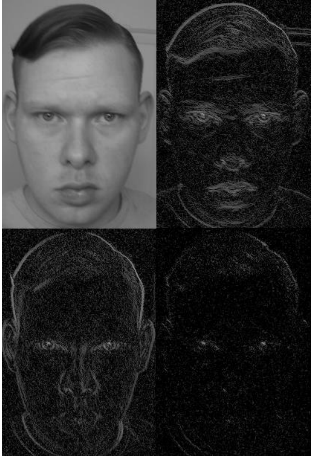
Figure 4.3 – Low frequency resultant blur output image (LL), high frequency horizontal edges sub-image (LH), high frequency vertical edges sub-image (HL), and high frequency diagonal edges sub-image (HH) derived from using a Haar wavelet transform on an input image.
