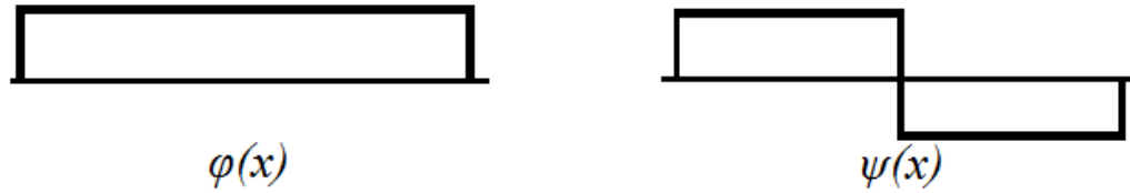
Figure 4.1 – Haar low pass scaling function \varphi(x) and Haar high pass wavelet function \psi(x) .
