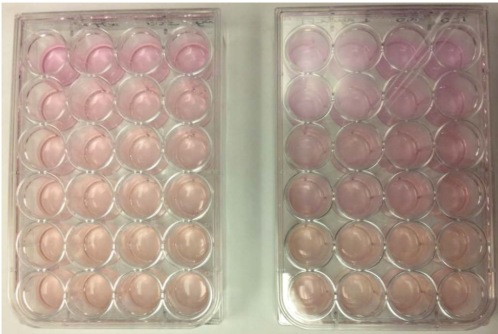
Figure 70: Unmilled magnesium supernatants after 24 h exposure to cells. On the left the supernatant prepared for 24 h and on the right the 1 week supernatant.
