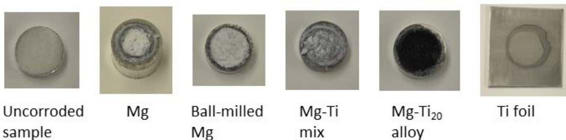
Figure 46: Sample surfaces before (far left) and after electrochemical corrosion experiments. Note the black surface on the alloy.
