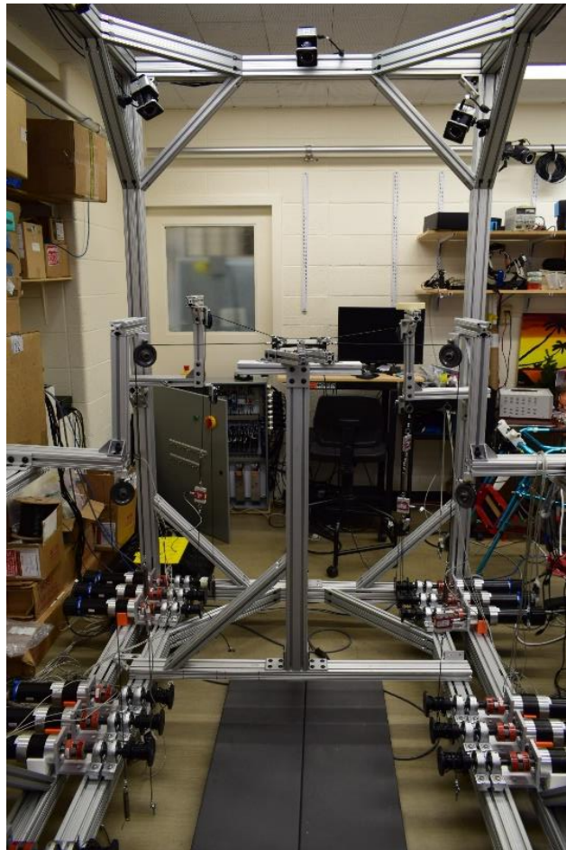
Fig. 5.6 Device setup for system validation. Acrylic plates are mounted to a force-torque sensor for measuring the external forces at the end effector.
