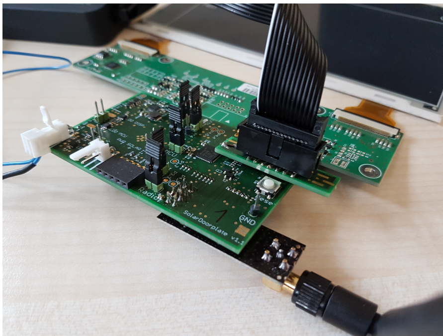
Figure 8.2: The Solar Doorplate circuit board stack: NRF24 transceiver (bottom), Solar Doorplate (middle), display controller (top), magnetic debug connector (ribbon cable)
