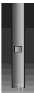
Figure1: Structural FE model with square-shaped opening at the height of half a meter from the ground
