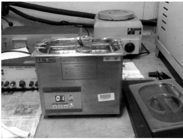
Figure 3: Sonication of nanofluid samples
