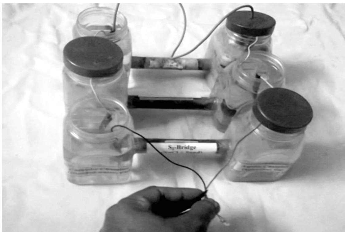
Figure 2: Bioelectricity generation by fuel cell
