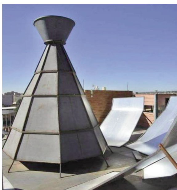
Figure 11: The addition of reflective mirrors to increase the amount of solar radiation.
