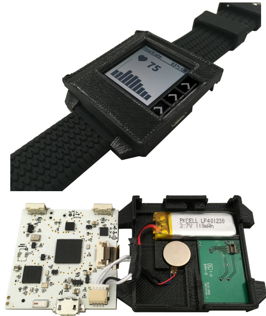
Figure 1: Perspective and interior views of our open-hardware wearable device, part of the open-source Amulet Platform. The platform supports development of energy-efficient, body-area-network sensing applications on multi-application wearable devices.
